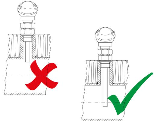
When using insulation, make sure that the immersion pipe is long enough.
