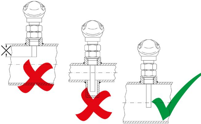
The measuring point must be in the middle of the pipe.
