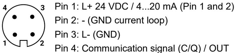
In addition to IO-Link communication, the pins are also used to supply the device.
